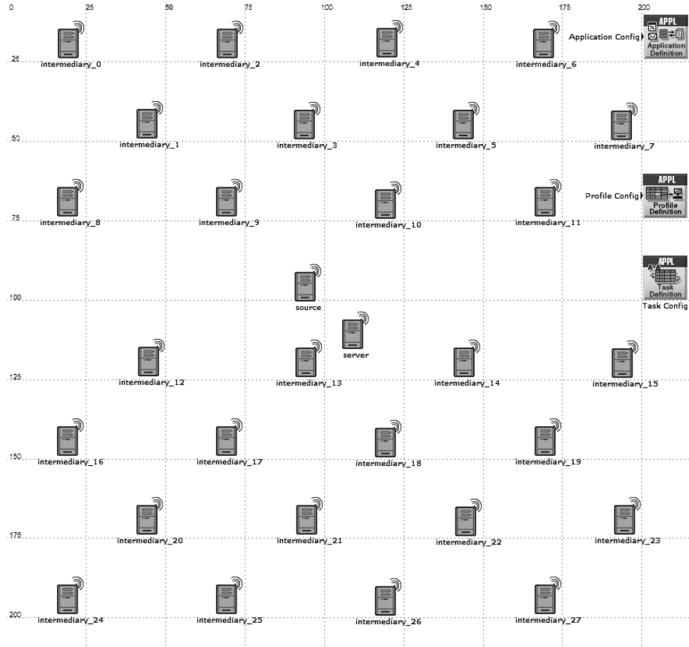
Figure 8.5: The network topology used in the simulation of the Chameleon protocol. There are 30 static devices distributed in a square area with 210 \times 210 meters. All devices are part of the set \Gamma of Chameleon users, and there is only one sender and one recipient in this scenario. The sender device is labelled source , and the recipient device is labelled server , and they are located approximately in the center of the topology. The three boxes located on the right hand side of the figure are used in the configuration and specification of the applications running in the simulation scenario. The Application Definition box is used to configure application parameters such as the transport protocol used and port. The Profile Definition is used in the configuration of the profile parameters to be applied to given application, such as the start time, duration, and repeatability of the service. The Task Definition is used for the configuration of the steps performed during the application run.
