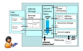
Figure 8. TPM-Based Attribute Handling on Terminal
